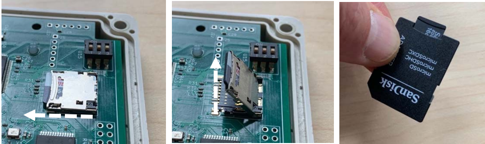
1. Slide Card holder 2. Lift SD Card holder up 3. Insert into Adaptor into PC 4. File Directory
